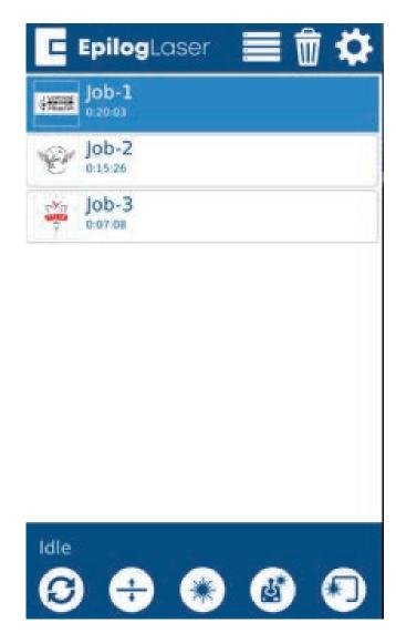
The **Job Menu** contains the **Main Buttons** that are used to control the laser. The two at the top of the screen are the **Job Menu** and **Delete.**
