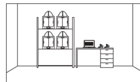
Multiple 3D printers in a large room, frequently printing parts in PLA Medium UFP concentration
